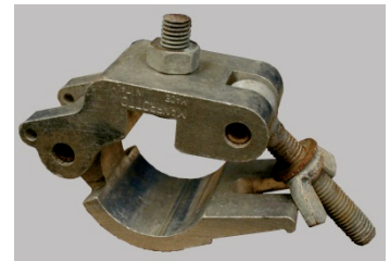
Fig.3 Half Couple Clamp for hanging the steel yoke
