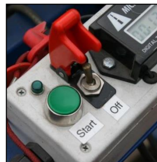
Fig. 4 On/Off Switch and Start Button
