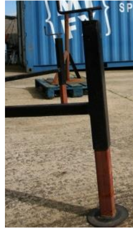
Fig 2. Outriggers secured at full length on the ground
