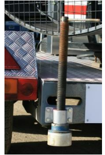
Fig 2. Trailer Feet in raised position
