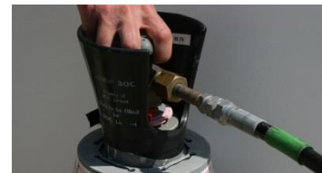
Fig.3 Turning on CO 2 Supply
