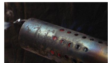
Fig.3 Coil heated to 'dull red', observed through cylinder holes
