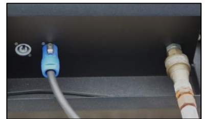
Fig 1. Power and gas connections
