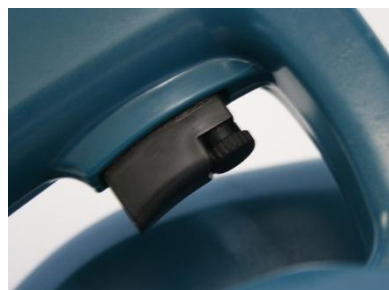
Fig 2. Trigger switch with speed control dial
