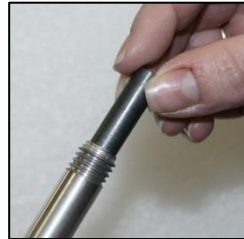
Fig 4. Insert flint into flint holder
