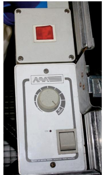
Fig.2 On switch and fan controller
