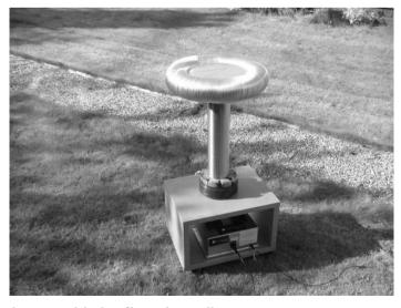
Figure 3. Correctly assembled coil on the trolley
