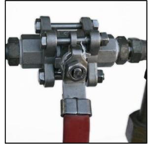
Fig 6. Valve closed
