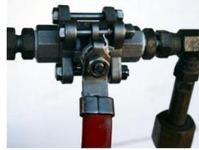
Fig 1. Valve Closed
