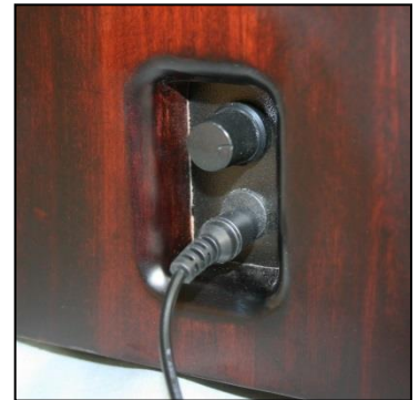
Fig 2. Power connection and control knob
