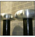
inside a Faraday cage or as part of 'Cage of Death' or 'Lightning Man' stunts. The SG100 outputs 1,00,000 volts to produce lightning bolts up to 2.5 metres in length – aimed towards the second SG100 as they are supplied as a pair. This item cannot be dry-hired.
