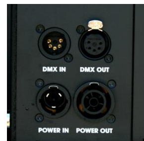
Fig 4. DMX & Power Sockets
