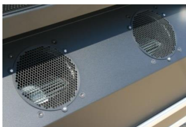
Fig 5. Close up of machine fans
