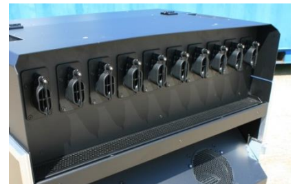
Fig 6. Close up of Bubble Blowers
