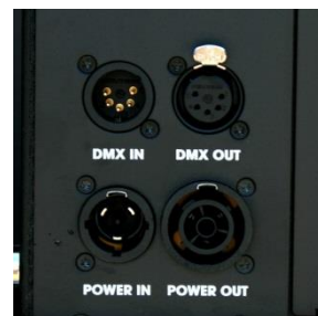
Fig 4. DMX & Power Sockets
