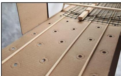
Fig 5. Removable base with perforated hole options
