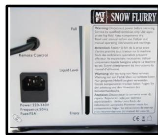
Fig 3. Fluid indicator & Power Connector
