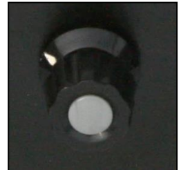
Fig 2. Flame height control
