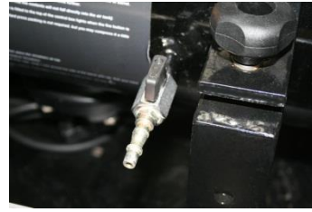
Fig.5 Air compressor connection
