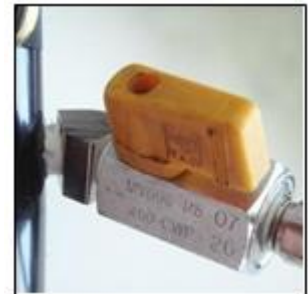
Fig 8. Filling lever in open position
