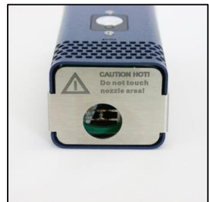
Fig 9. Smoke output, caution - hot
