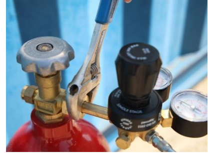
Fig 7. Fastening CO2 to regulator & gas hose
